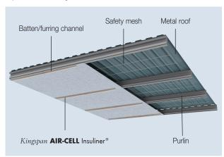
Figure 3 Warehouse metal deck roof retrofit installation
