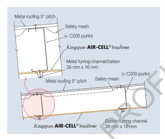
Figure 4 Side elevation of Kingspan AIR-CELL Insuliner® in a warehouse metal deck roof retrofit
