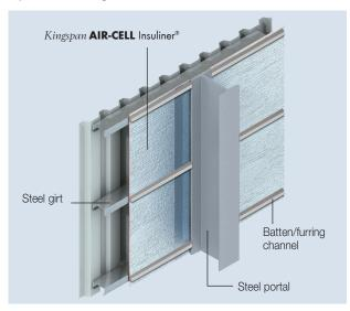
Figure 7 Warehouse wall retrofit installation
