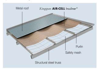
Figure 1 Warehouse metal deck roof installation
